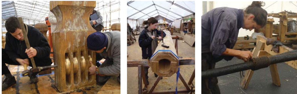
L'Hermione : under construction; working on the pulleys, masts and ropes
